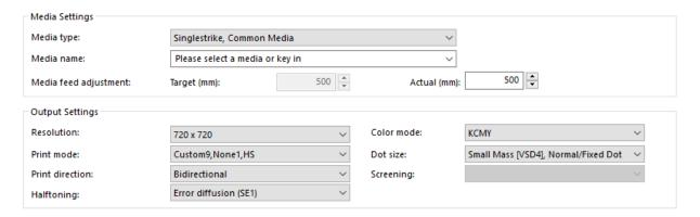
The "Resolution", "Print mode", and "Dot size" settings are linked. Each time you select a different resolution, the appropriate print mode and are dot size are displayed.
